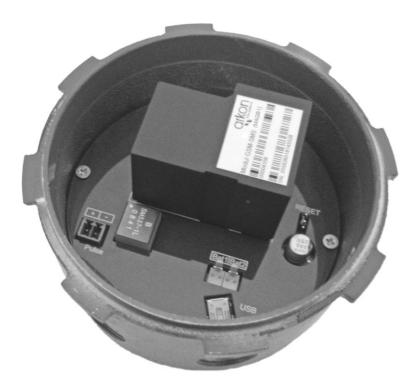
Picture 3. Install 3G/GPRS/GSM Module into the transmitter
