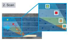
By correlating/comparing the saved signals, the positions of unambiguously identifiable reflectors can be identified. The reflectors can be identified at varying positions within the images since they have moved with the medium.
