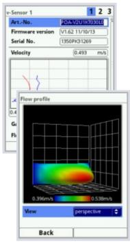
The NivuFlow 750 uses up to 9 x 16 gates for flow measurement.
