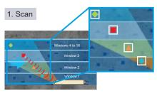
A few milliseconds later a second scan follows. The resulting echo patterns are saved as well.
