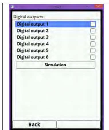
Fig. 7-101 Display status of digital outputs
