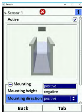
Fig. 23-17 Sensor installation direction altering options
