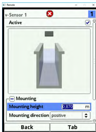
Fig. 23-16 Setting the mounting height
