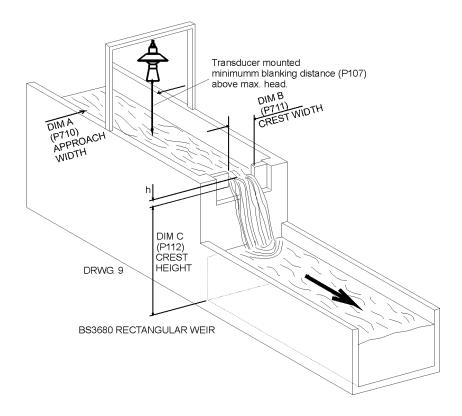
In this example it is required to calculate to the flow through a BS3680 Rectangular weir. Absolute calculation will be used, and there is a requirement for an alarm to indicate a high flow condition to be set to relay 3. The flow rate is required to be displayed in litres/minute and the totaliser is to record the flow in cubic metres, the resettable totaliser is to be displayed during RUN.
