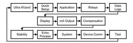
As you press the cursor keys to scroll left and right between these, you can press ENTER at any time, to select the desired menu heading, and take you to the sub-menu.
