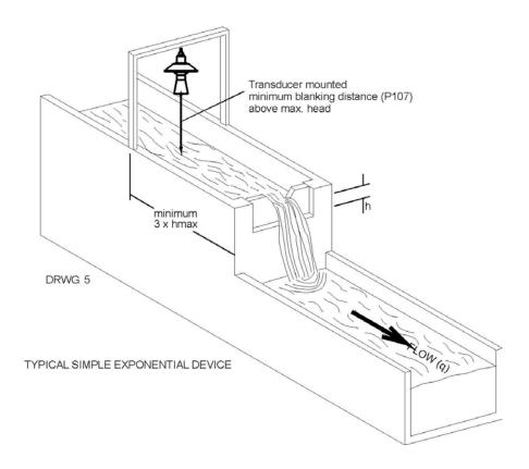
In this example it is required to calculate the flow through a Simple Exponential Device, which on this occasion is a V-Notch Weir. The K factor for the weir is unknown so ratiometric calculation will be used, there is no requirement for alarms and the flow rate is to be displayed in litres/second. The totaliser is to record the flow in cubic metres but is not to be displayed during RUN.
