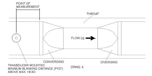
When any **Other** device is chosen please consult the manufacturer of the device for details of where the point of measurement should be located but ensure that it is chosen such that the surface of the liquid is not effected by turbulence or drawdown.
