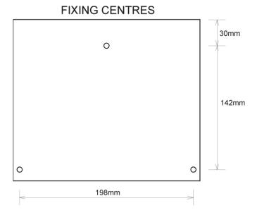
The *NivuMaster* should be mounted by drilling three holes suitable for size 8 screws (length to suit your application), and fixing the top screw in place. Hang the unit on this and fix the two remaining screws by removing the terminals access cover to access the pre drilled holes.
