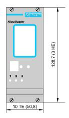
Dimensions of the panel enclosure are as shown below:
