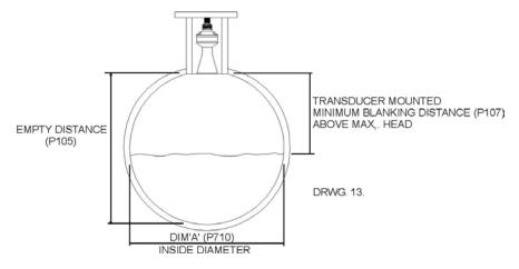
If the flow calculation is to be **absolute P702** = 1 the flow will be calculated using the formula: q = va(h)
