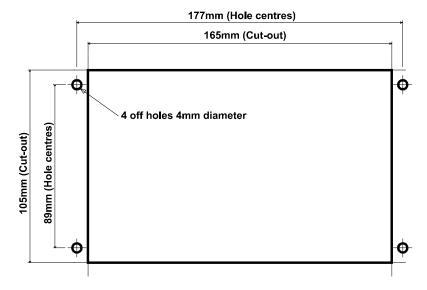
The full dimensions of the Panel mount enclosure are as shown below.
