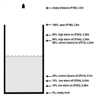
In this example, there is a pump (relay 1), which will come on if the level rises to 2.24 m, and go off when the level drops to 0.7 m. (**control down**). If the level rises to 2.4 m, then the high level alarm (relay 4) will come on until the level drops to 2.24 m. If the level falls to 0.28m, then the low level alarm (relay 5) will come on until the level rises to 0.42 m.
