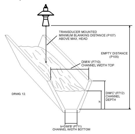
If the flow calculation is to be **absolute P702** = **1** the flow will be calculated using the formula: q = vh (b + mh)
