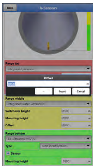
Fig. 36-12 Programming integrated pressure sensor
