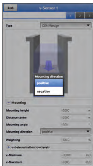
Fig. 36-19 Modifying the sensor mounting direction
