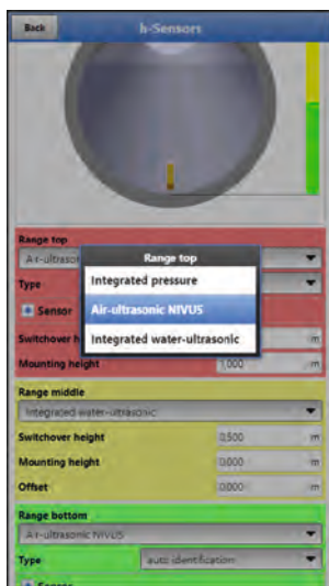
Fig. 36-11 Level sensor assignment to programming section
