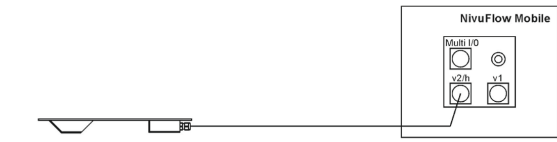
Fig. 25-2 Connection of level sensor DSM-L0
