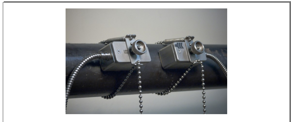
Illustration 6: Sensor mounting with clips and chains
